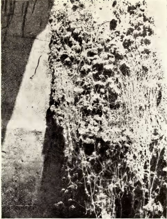
Fig. 1. Fouling of copper sheathing above the bilge-keel. (Portion on the left has been scraped, exposing copper plates.)
